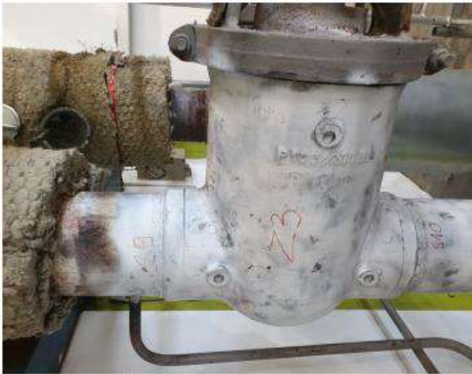
Fig.7. Example of cleaning preparation for MT testing of V – valve.
