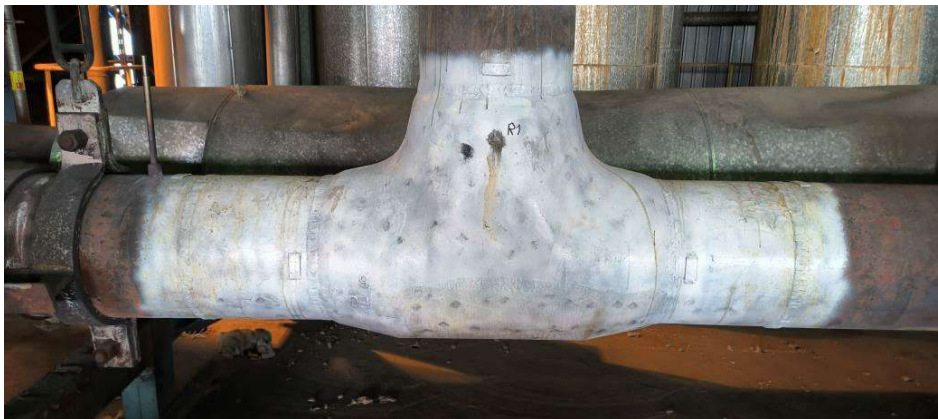
Fig.4. Example of cleaning preparation for MT testing of tee – surface and welds
