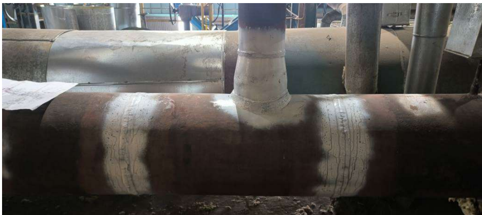
Fig.5. Example of cleaning preparation for MT testing of tee – and welds
