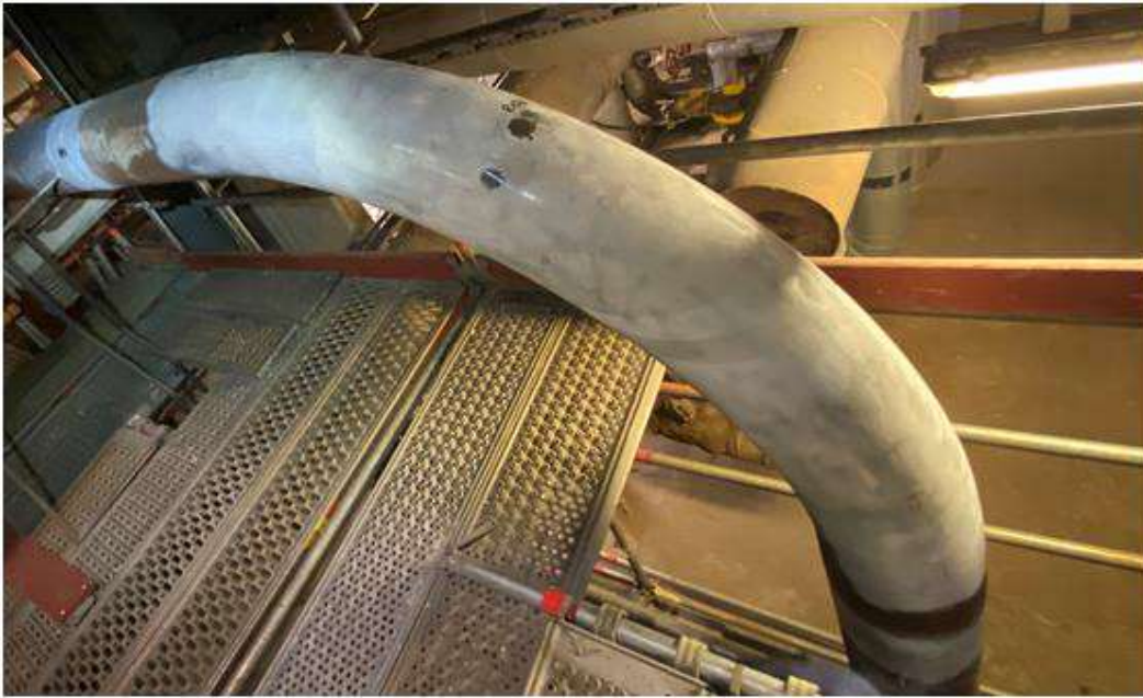
Fig.3. Example of cleaning preparation for MT testing of elbow – surface and welds
